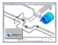
**SINETZ** is the design solution for Steady State Calculation of Flow Distribution, Pressure Drop and Heat Loss in Branched and Intermeshed Piping Networks for compressible and incompressible media.
